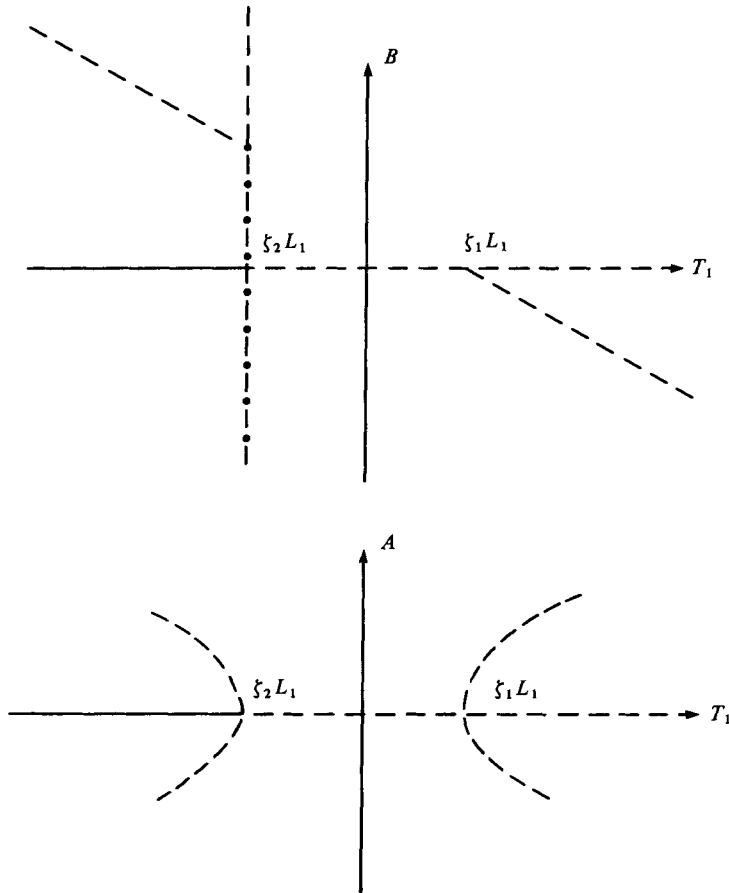
FIGURE 3. The solutions of (3.10) for  $L_1 > 0, f_1 = f_2 = 0$ . —, stable solutions; ····, neutrally stable solutions; ---, unstable solutions.
