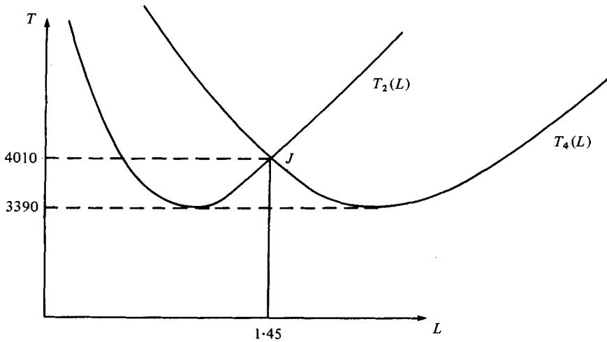
FIGURE 2. The neutral curves for the two-cell and four-cell modes.
